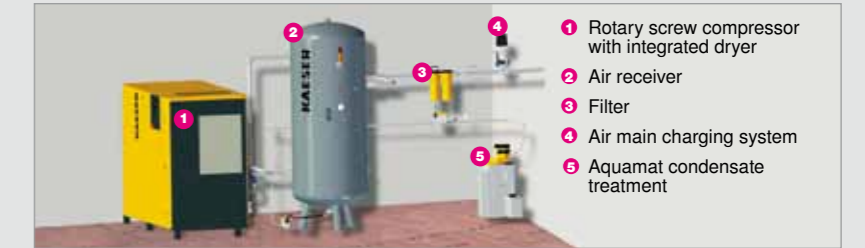
Compressed air supply system with T-version compressor
