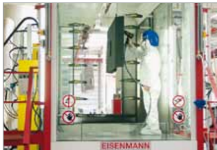
The machines get their tough paint finish in the powder-coating installation
