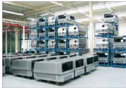
Enclosures for the portable compressors
