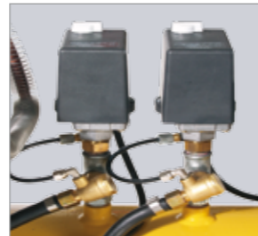
Dual pressure switches Dual pressure switches vent the compressors for unloaded starting. The cut-in and cut-out pressures can also be individually set.
