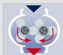
Conveying to discharge side
