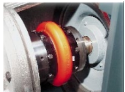
Fig. 3: On real one-to-one drive, only a coupling is fitted between the drive motor and the air end. This is why there are no transmission losses between these components.
